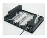
The thinXXS flow sensor module, developed through collaborating partners of the microBuilder Consortium, consists of two silicon flow sensor chips, read-out electronics with analogue and digital output and polymer packaging containing standardized fluidic
